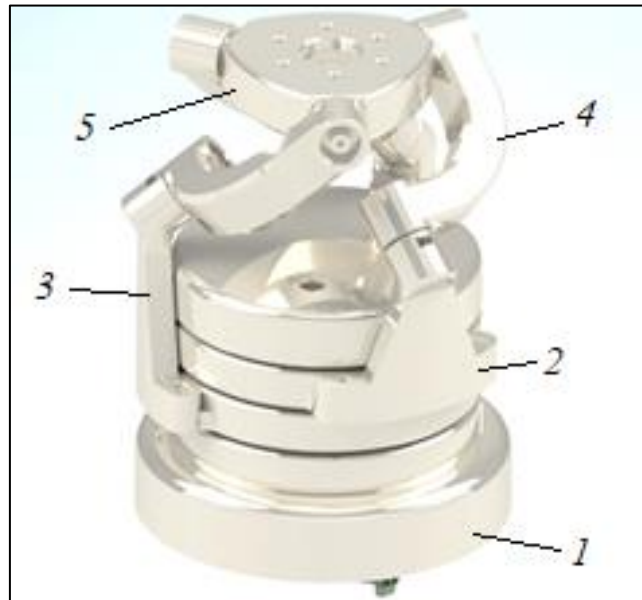
Fig 1: The structure of a 3-DOF spherical parallel manipulator with a 3-RRR and coaxially actuated input joint: 1-Base; 2-Rotary plate; 3-Proximal link; 4- Distal link; 5- Wrist.
