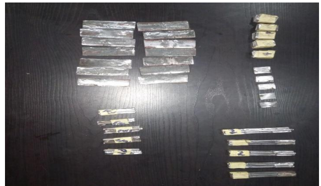
Fig 5: HSLA Samples for Mechanical tests after welding, cutting and PWHT
