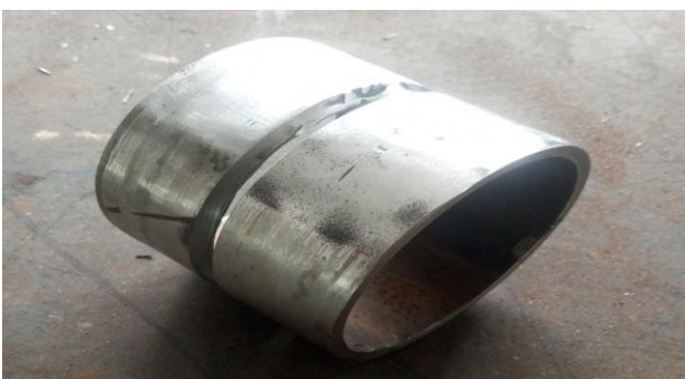
Fig 3: Two sections of the HSLA sample material tacked together before root pass welding
