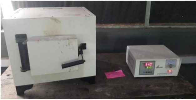
Fig 6: The Muffle Furnace used in PWHT
