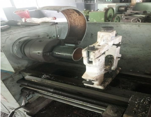
Fig 1: Preparation of the HSLA sample material on a lathe
