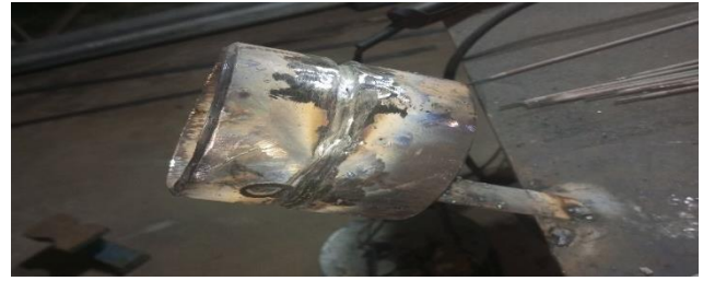
Fig 4: Sample material welded in 6G position after hot pass welding
