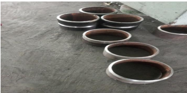
Fig 2: Cut sections of the pipe material before welding
