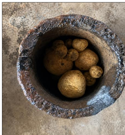
Fig 1: Gold ores loaded in a crucible ready for smelting; spheroidal ore masses of varying sizes prepared for the furnace (Researcher's photograph, 2024)
