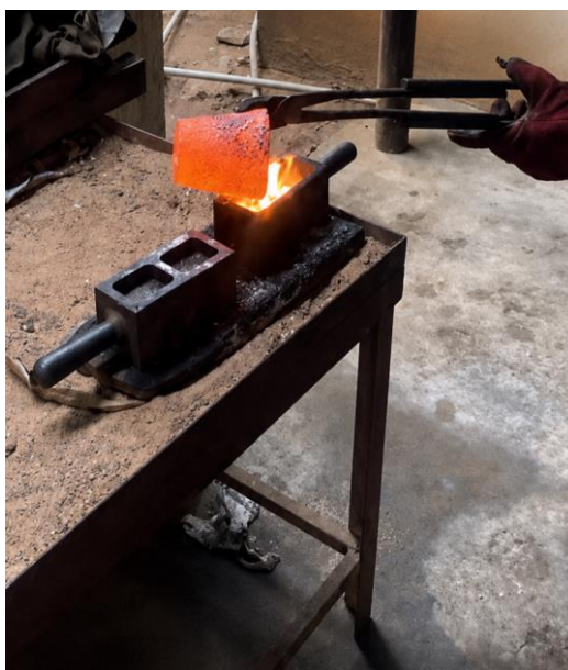
Fig 6: Pouring molten gold from a crucible into an iron ingot mould, showing the incandescent orange stream of liquid gold and the two-cavity mould configuration used in small-scale operations (Researcher's photograph, 2024)
