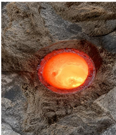
Fig 5: Smelted gold in a crucible as removed from the furnace, showing the characteristic incandescent orange-white glow of molten gold at approximately 1,100°C surrounded by slag residue (Researcher's photograph, 2024)
