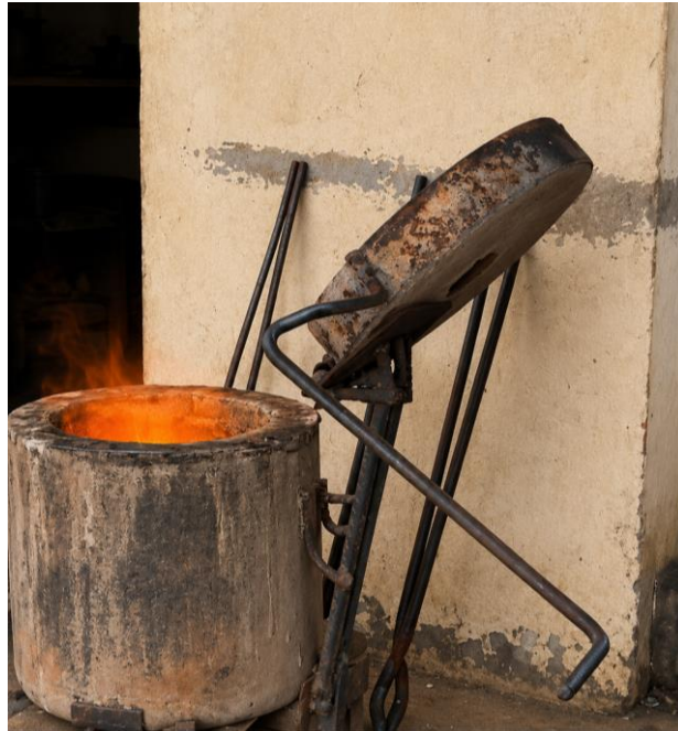
Fig 3: A traditional smelting furnace at a small-scale gold processing site in Ghana, showing the refractory crucible vessel at high temperature with tongs and crucible-holding frame alongside (Researcher's photograph, 2024)
