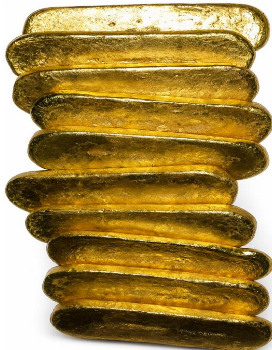
Fig 8: Stack of completed gold bars produced by small-scale smelting operations, showing the characteristic form, surface texture, and golden colour of artisanal gold bars following smelting, casting, and acid pickling (Researcher's photograph, 2024)
