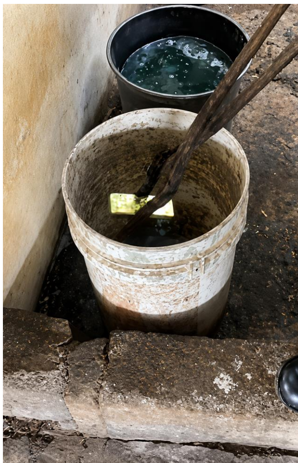
Fig 7: Acid pickling of a gold bar in a dilute acid solution, with the immersed bar visible at the bottom of the container alongside tongs used for handling — the dark green solution indicates the presence of dissolved copper and base metal impurities (Researcher's photograph, 2024)
