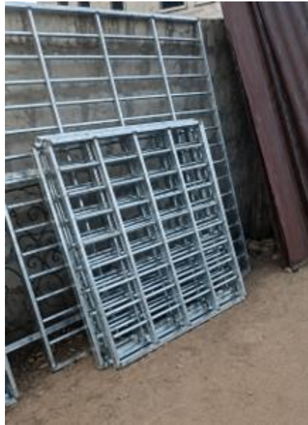
Fig 9: Completed, galvanised steel window-guard and security panels, fabricated from welded angle-iron and bar-stock frames, awaiting installation.
