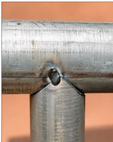
Fig 5: Fillet weld at a T-branch pipe connection.
