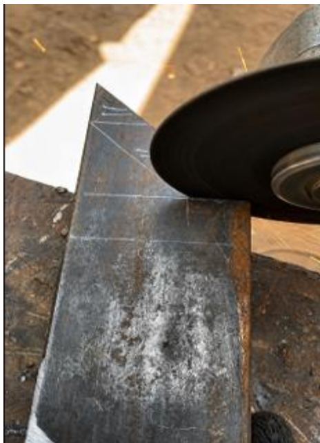
Fig 1: Marking-out and abrasive grinding of a 45° mitre bevel on mild steel angle iron.
