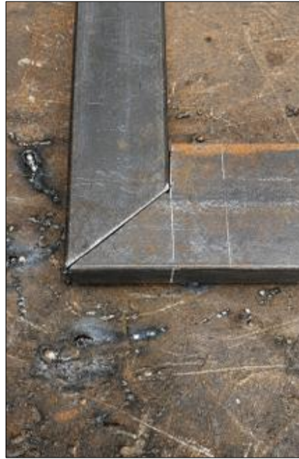
Fig 2: Mitre corner joint of angle iron prior to welding.
