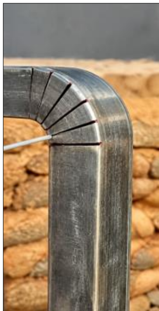
Fig 7: Close-up of a segmented (kerf-cut) bend in square tube. Wedge-shaped relief cuts have been made at regular intervals to allow the tube to be curved.
