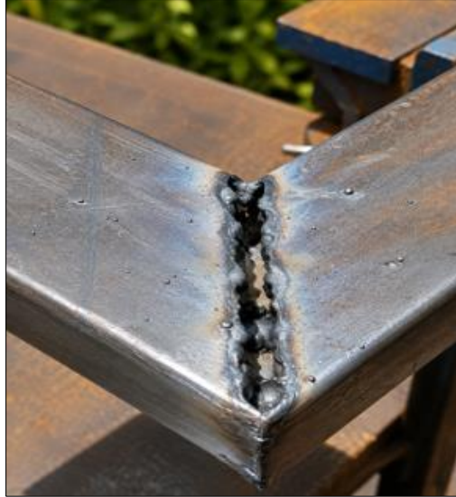
Fig 4: Close-up of a finished mitre corner weld on angle iron showing surface porosity (rounded voids along the weld bead) and an incompletely fused root gap.
